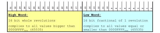
Now the scaling of the analogue output can be set in a way, that the maximum output voltage range of +/- 10V can be used for a position range smaller than 1 revolution. To do this the scaling for the output has to be set in the input field "Scaling" of the window "Analogue outputs" of the ServoCommander<sup>TM</sup> software.
